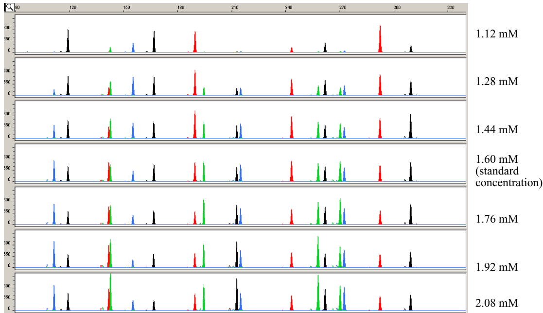
Figure 6-1 1 ng genomic DNA amplified with the AmpFSTR Yfiler Kit in the presence of varying concentrations of magnesium chloride: 1.12 mM, 1.28 mM, 1.44 mM, 1.6 mM, 1.76 mM, 1.92 mM and 2.08 mM, analyzed on the ABI PRISM 3100 Genetic Analyzer
