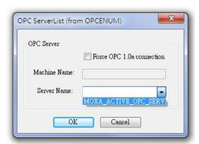
If the Active OPC Server Lite is installed on a remote PC, select **Connect** → **Remote** from the menu bar. Input the host name (i.e. Moxa\_Client) or IP address and specify **MOXA ACTIVE OPC SERVER** in the **Server Name** column.
