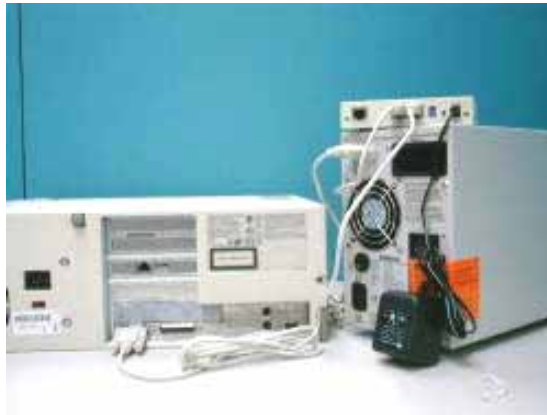
Figure 2-4 Serial cable connection of USHA ProE II
