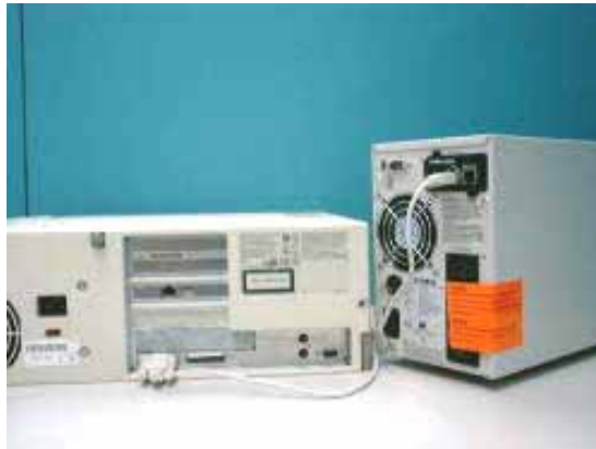
Figure 2-3 Serial cable connection of USHA Pro II (mini USHA)
