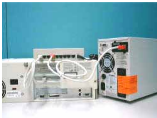
Figure 2-19 Connecting the Ethernet cable from the LAN port of USHA Pro II and mini USHA.
