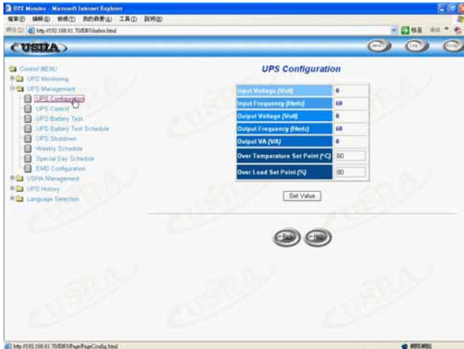
Figure 3-8 USHA UPS Configuration screen
