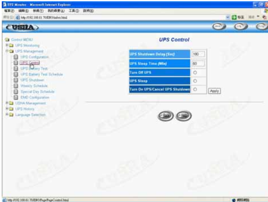
Figure 3-9 USHA UPS Control screen
