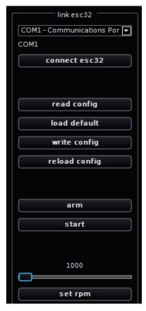
Connect UART adapter to ESC32 and computer and choose the UART adapter you are using and click connect.
