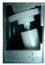
The thermostat inside the machine is for chill mode only and has no effect on machine when on slush mode.
