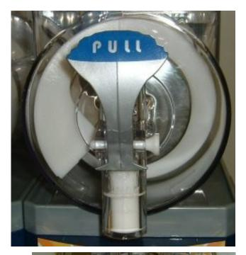
Push dispensing plunger up to remove handle. Remove plunger and spring.
