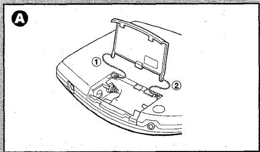
Open the battery compartment and insert two size AA (LR6) alkaline batteries with the  $\oplus$  and  $\ominus$  marks correctly aligned.
