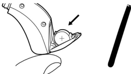
If the battery drawer does not close easily, the battery is incorrectly inserted.
