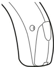
Close the battery drawer to turn on the hearing aid. An acoustic indicator will indicate that the hearing aid has been switched on unless this function has been disabled.
