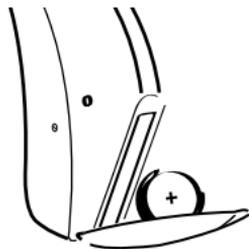
When the hearing aid is not in use, the battery drawer should be left open, to ventilate the hearing aid and allow it to dry.
