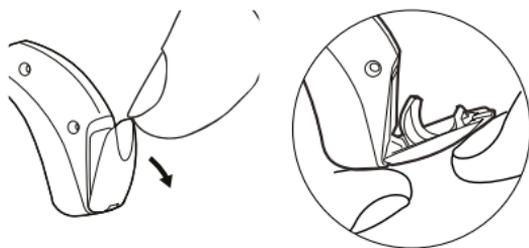
Place the battery in the drawer as illustrated, so that the plus (+) sign on the battery is facing towards you when you hold the hearing aid as shown. You can use the battery magnet provided to steer the battery into place.
