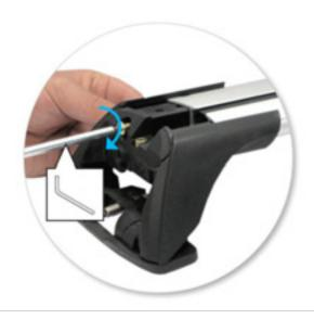
Tighten adjusting screw to 5 Nm.
