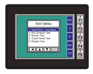
Serial Port - Loop Back Test - Performs a test to verify either the RS-232 or the RS485/422 serial communications functionality from the 15-pin connector (Port 2) on the panel is operating correctly. A loop back connector inserted into the port is required for proper testing. Wiring diagrams to build RS-232 and RS-485/422 loop back connectors are shown below.
