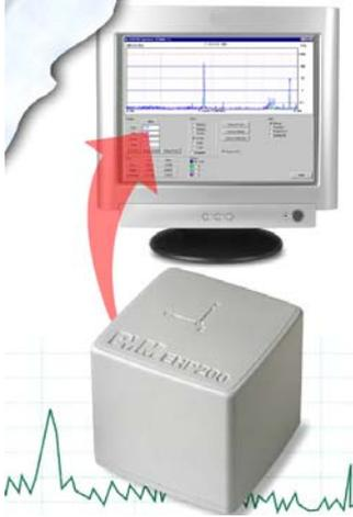
EHP-200/A E-H fields analyzer has been designed for accurate measurements of both electric (0,02 to 1000 V/m) and magnetic (6 mA/m to 300 A/m) fields, in the frequency range 9 kHz to 30 MHz.
