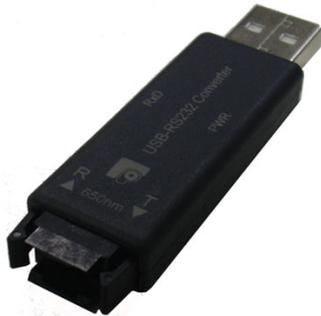
USB-OC is an standard accessory of the EHP-200/A Analyzer. It converts the signals of some of the system's accessories, which are only connected via fiber optic, into USB-compatible signals. It, therefore, makes it possible to link the following items up to the USB port of any Personal Computer to operate them in conjunction with specific application software and for firmware updating:
