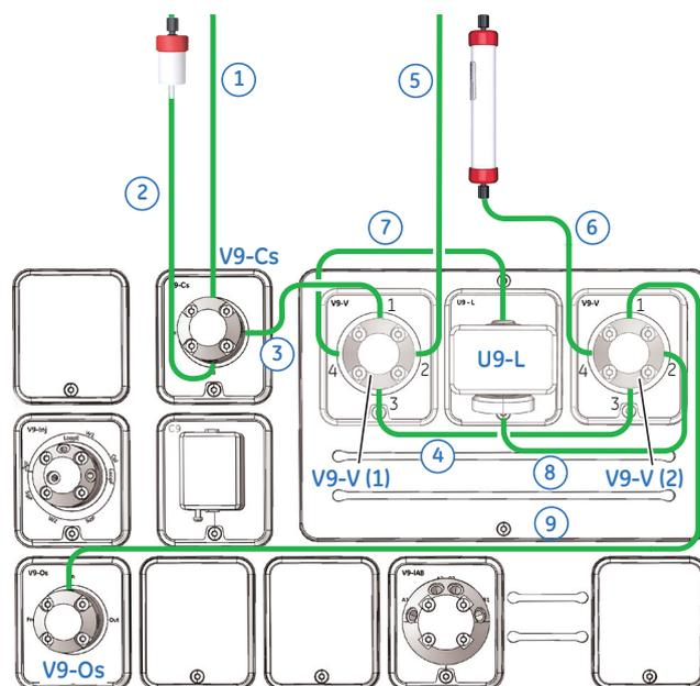
The illustration shows the flow path allowing tandem two-step purification using the UV monitor **U9-L** installed on ÄKTA pure<sup>1</sup>.
