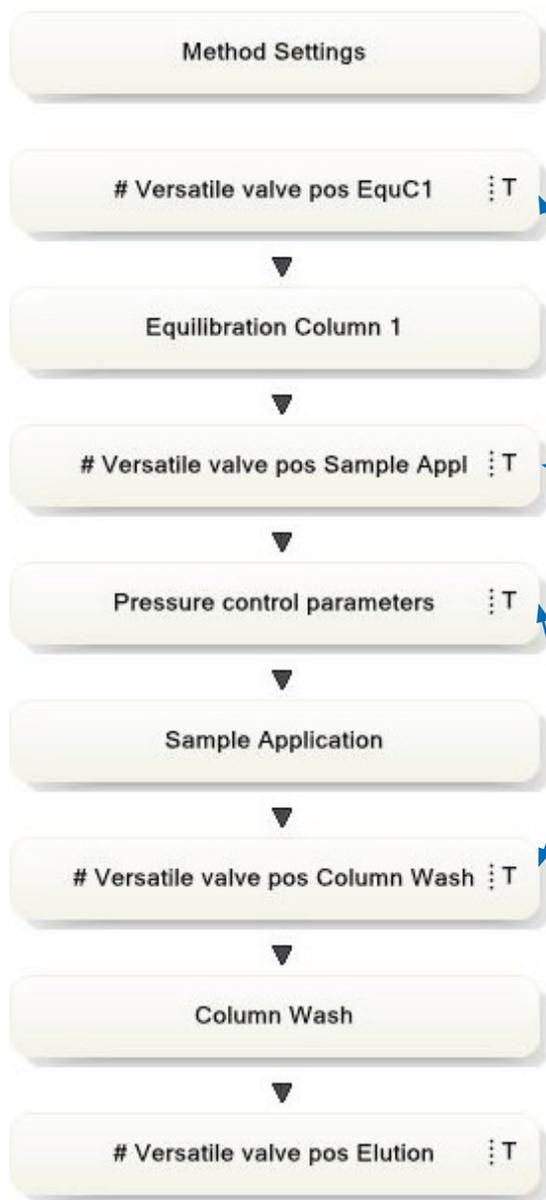
User defined phases to set the valve configuration to the Wash and Elution steps.
