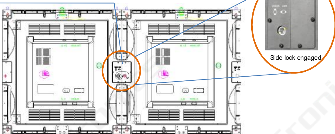
Image 4-3 Two tiles horizontally connected with side lock
