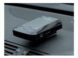
Note: 3Zero may not work in vehicles with a heat reflective windscreen. If your vehicle has this type of screen, look for a clear area to mount the unit such as by the rear view mirror.
