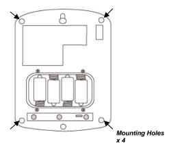
Before Installation, refer to your Control Panel manual to temporarily disable the Siren Tamper function to avoid accidental alarm trigger.
