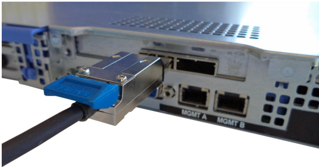
Connecting the SAS Cable to the Bridge SAS Port
