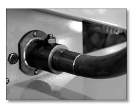
If necessary swap the cable and support to the opposite end of the machine table (Pull hard to remove the cable from the socket on the side of the machine).
