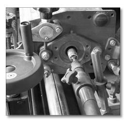
Connect the flexible reel drive to the cutting head using an appropriate drive adaptor.
