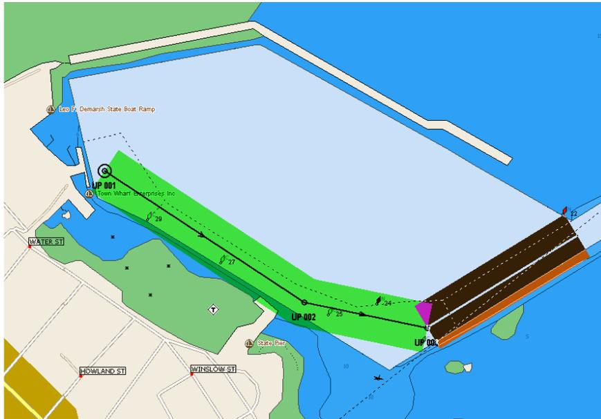
In the image above, the area shaded in green has been 'route checked' by PC-Planner for all hazards defined on the Route Checking tab. The black area is where the new leg of the route is being drawn. The shading allows you to see the area being checked and it is defined by the Width setting on the Route Checking tab.
