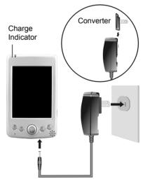
3. The charge indicator glows amber when charging is in progress. Do not disconnect your Pocket PC from AC power until the battery is fully charged, as indicated by the amber indicator turning into green. This will take a couple of hours.
