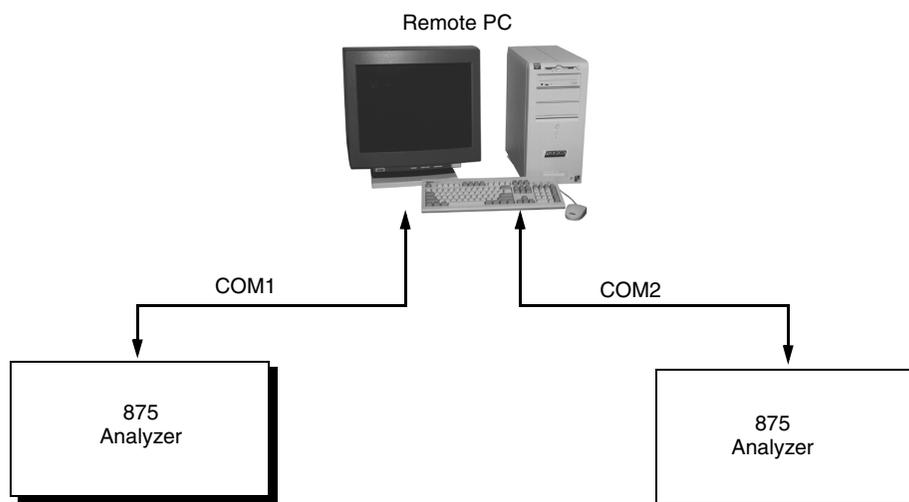
*Figure 1. External Interface between a Remote PC and Two 875 Analyzers*
