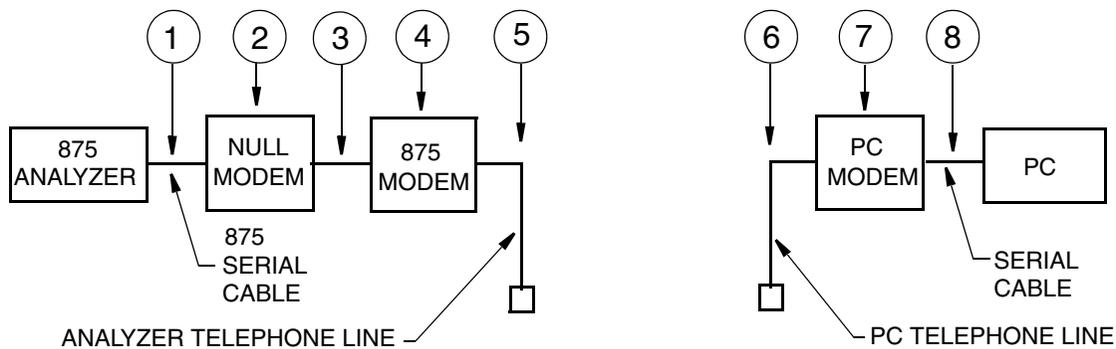
*Figure 8. Required Equipment for Operation With Modems*
