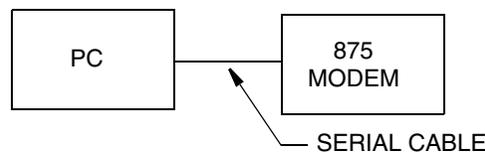
*Figure 9. Connections for Configuring the Analyzer Modem*
