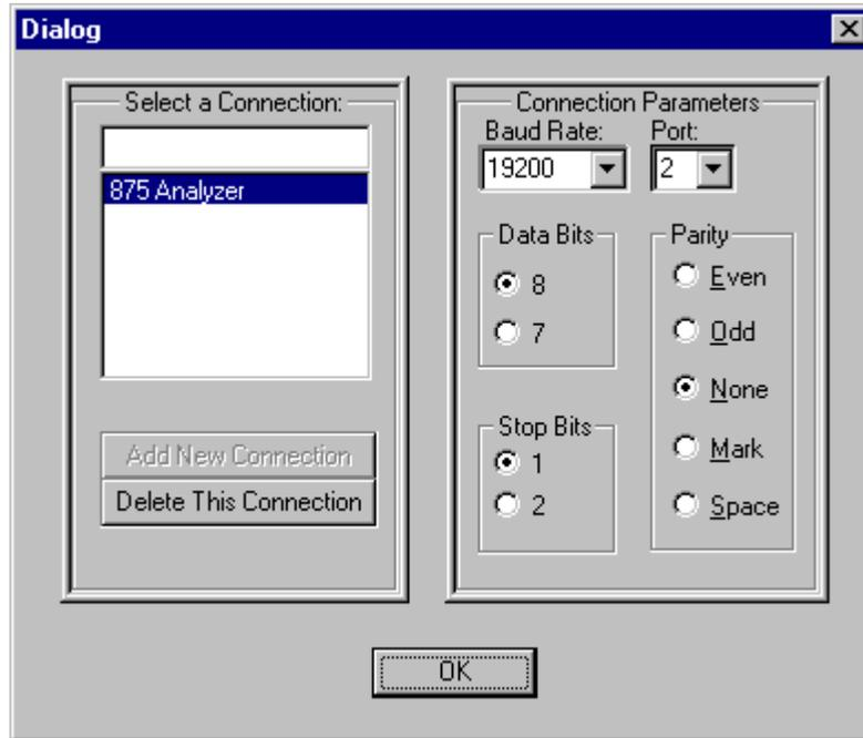
*Figure 3. Connections Parameter Screen*
