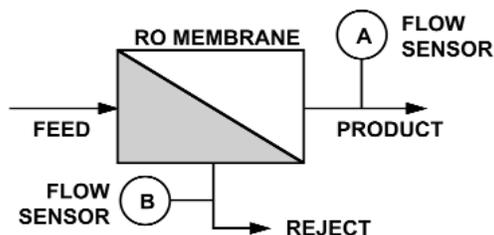
Channel A secondary measurement can be % recovery
