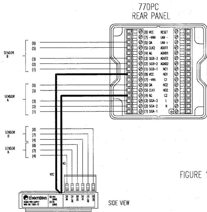
FIGURE 1. 24VDC-Powered Sensor Connections
