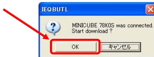
**Caution** Do not turn off the power to the QB-78K0SKX1-DA nor disconnect the USB interface cable from the QB-78K0SMINI during downloading; otherwise, it will not be possible to restart the QB-78K0SMINI.
