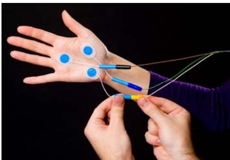
**Figure 4-2** Correct way of disconnecting the electrodes
