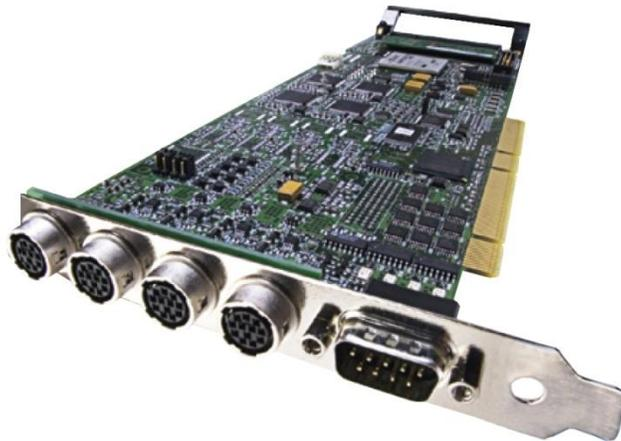
**Figure 6-4** PCI X Bus Frame Grabber
