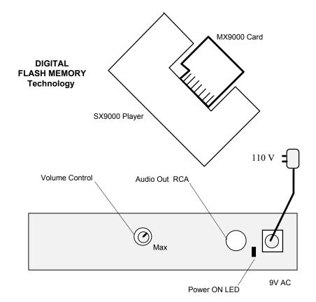
Audio playback starts automatically as soon as the power is connected, the Green LED light turns On to indicate the device is ON and is playing.
