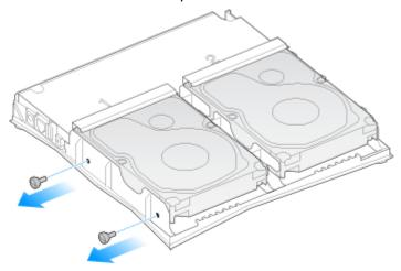
**4.** Pull the disk forward to disconnect it from its plug and then lift the disk up to remove it from the enclosure.
