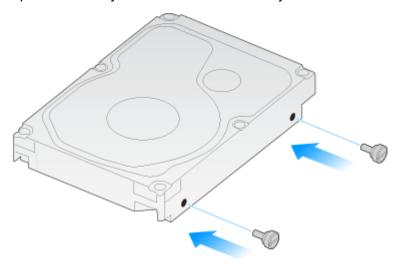
2. Guide the hard drive so that the rear screw fits into its slot, and then slide the drive into its plug.
