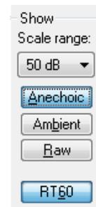
RT60 shows the amount of time for the sound pressure level to decay 60dB. This is a standard method to evaluate the decay time of a room.
