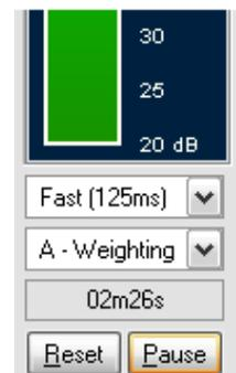
The second menu allows for switching between the weighted frequency curves:
