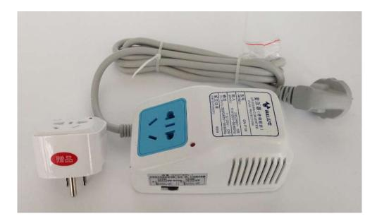
This is an extra part for countries using 110V AC. Turn table only functions at 220 V AC. Countries using 110V AC can use this adaptor to switch the voltage. This is a temporary solution. There will be a voltage transmitter built within the turn table later on.
