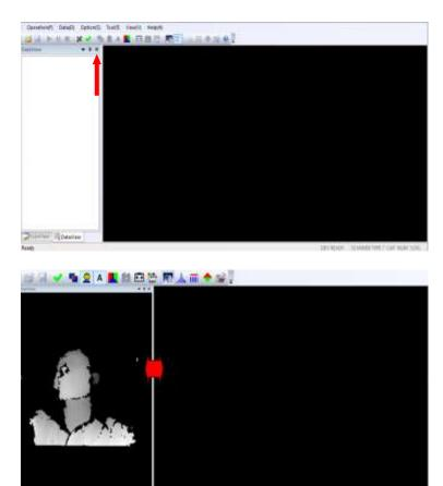
Close the data window to show the scanned view. If there is object appearing 40cm in front of the infracted sensor, the left hand side window will show modeling at real time bases. If window is too small to show the full image, drag the side of the window to enlarge.
