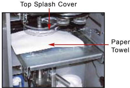
25. Place a cloth or paper towel on the turntable (under the top splash guard) to collect polish during hose priming.
