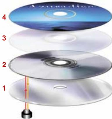
1. A disc is created from molten polycarbonate and digital information is stamped on the top of the disc, while it is still near melting point, using a die with microscopic bumps. These bumps are known as "pits and lands".
