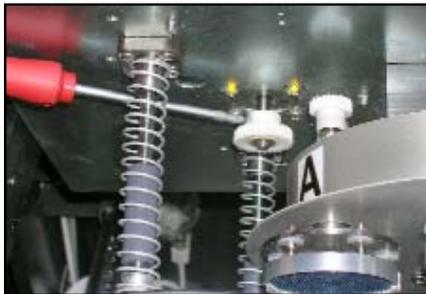
5. Using a #1 Phillips screwdriver, remove the lock screw from the Polish Head Motor drive gear.
