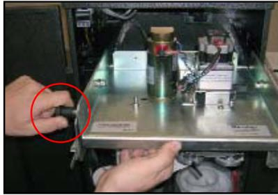
2. Pull drawer out. Pull knob on left side of drawer out. While holding knob out, slowly lift drawer up and rotate back. Release knob into place.
