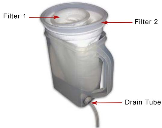
9. Verify that Filter 1 is inside Filter 2 and both filters are in the Water Pitcher.
