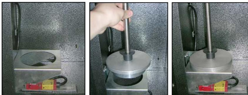
4. Ensure that the Plastic Lift is properly installed (T-side up) on both Spindles.
