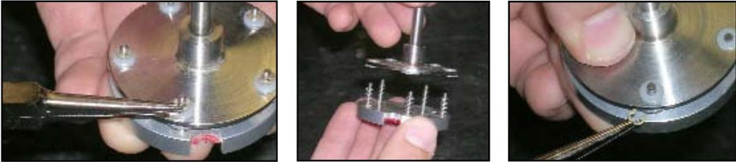
6. Remove retaining clips using needle nose pliers, replace polish head and reinstall retaining clips.
