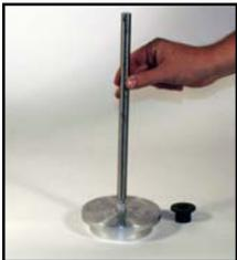
Step 1. Screw the shaft onto the threaded base. The adjustable nut is the white nylon collar just below the shaft threads.
