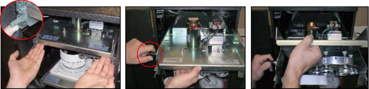
1. Lift both Release Tabs and pull out the Polishing Pad Turret Drawer.
