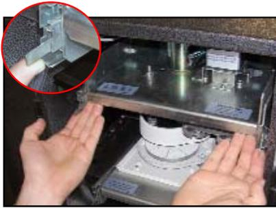
1. Lift both Release Tabs and pull out the Polishing Pad Turret Drawer.
