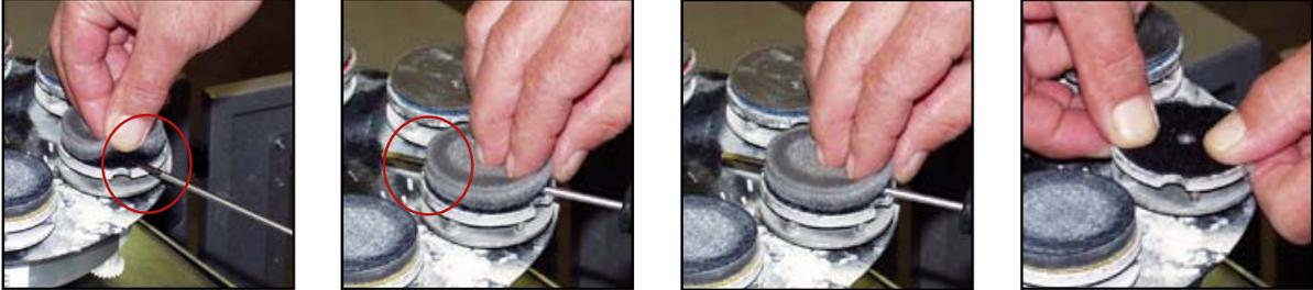
3. Carefully lift the edge of the Polish Pad and insert the tip of a small flat screwdriver between the "hook and loop" fastener as shown.
