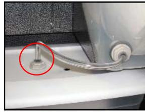
10. Verify that Drain Tube is secure in the Water Tank Cover quick disconnect fitting.
