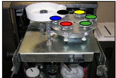
16. Place pads on heads according to velcro color code. Ensure the pads are centered on the heads.
