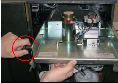
14. Pull drawer out. Pull knob on left side of drawer out. While holding knob out, slowly lift drawer up and rotate back. Release knob into place.
