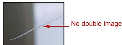
Top side foil dents are not scratches but look like a scratch on the reading side of the disc. The dent is made by a large amount of pressure put on the label side of the disc, causing the foil layer to dent. This dent will cause skips and cannot be repaired, however they can be prevented using an Azuradisc Scratch Guard.
