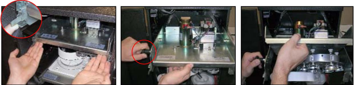
1. Lift both Release Tabs and pull out the Polishing Pad Turret Drawer.
