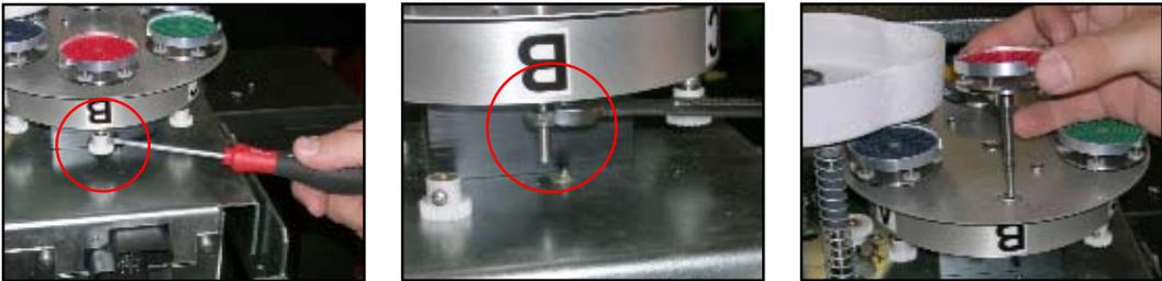
3. Using a #1 Phillips screwdriver, remove the small screw from the small gear.
