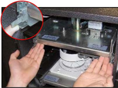
13. Lift both Release Tabs and pull out the Polishing Pad Turret Drawer.
