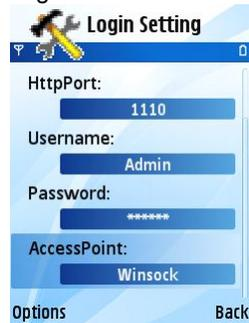
**Step8** : Input the server's address, ID and password respectively. Then save.
