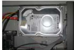
**Fig 2.1 Connect HDD**
