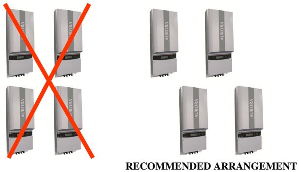
Fig.7 Recommended installation of AURORA inverters
