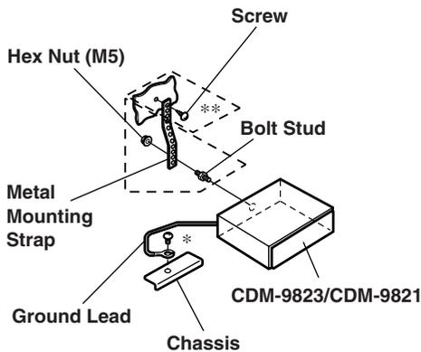
Reinforce the head unit with the metal mounting strap (not supplied). Secure the ground lead of the unit to a clean metal spot using a screw (\*) already attached to the vehicle's chassis.
