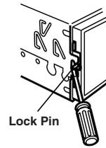
Slide the CDM-9823/CDM-9821 into the dashboard. When the unit is in place, make sure the locking pins are fully seated in the down position. This can be done by pressing firmly in on the unit while pushing the locking pin down with a small screwdriver. This ensures that the unit is properly locked and will not accidentally come out from the dashboard. Install the Detachable Front Panel.
