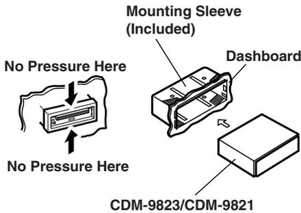
Remove the Detachable Front Panel (refer to page 4). Slide mounting sleeve from main unit. (see "Removal" on this page). Slide the mounting sleeve into the dashboard.
