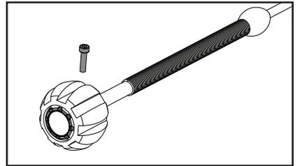
**To attach either probe-centering brush set**, identify the end with three set screws. Passing the camera head through the *other* end first, slide the probe through the brush set until the camera head protrudes 1/8 in. past the end with the set screws (see figures below). In this position, the three set screws will line up with the head's Accessory mounting ring. Secure the brush set to the head by hand-tightening the screws.
