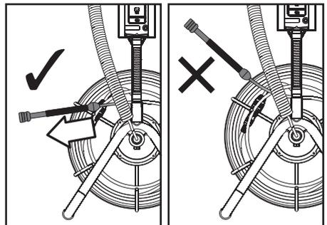
Once you have played out a few feet of probe, lock the reel by fastening the Velcro closure around the reel frame, as shown below at right.
