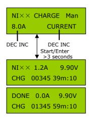
In "Man" mode the 680B+ charges the battery using the current you set on the second line.
