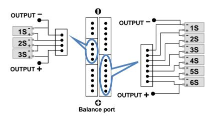
Balance port includes 5 connectors which are connected to 2S, 3S, 4S, 5S or 6S battery with XH balance connectors separately. For Thunder power, Flight power and Polyquest, Hyperion battery, please through adapter board CCB-7TPQF connecting the charger and battery, and the CCB-7N-EH is for the Kokam battery.
