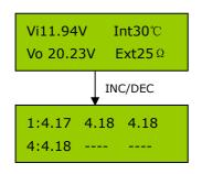
On the top line, Input voltage and Internal temperature are displayed And the bottom line, Output voltage (connected battery voltage) and external temperature are displayed
