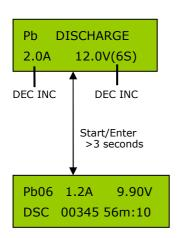
Set the discharge current and the nominal voltage of the battery. The discharge current ranges from 0.05 to 7.0A. The voltage should be matched to the nominal voltage of the battery to be discharged. The nominal voltage range is 2-24V.
