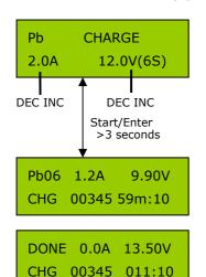
Set the charge current and the nominal voltage of the battery. The charge current range is  $0.05\sim10.0A$  and should be set to 0.1C for the battery to be charged. The voltage should be matched to the nominal voltage of the battery to be charged. The voltage parameter range is 2-24V(1-12S).
