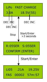
On the left side of the first line, You can set up the type of battery (LiPo, LiIo, LiFe). The values on the second line set the charge current and the voltage (cell count) of the battery pack. Press **START/ENTER** to make the value flash then press **DEC** or INC to adjust the value. After setting the current and voltage press START/ENTER again for more than 3 seconds to start the process. (Charge current: 0.05~10.0A, Voltage: 1~6 series)
