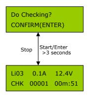
The left screen is displayed when the charger detects the battery voltage in the CHARGE or FAST CHARGE mode.
