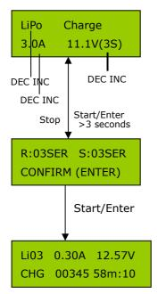
On the left side of the first line, You can set up the type of battery (LiPo, LiIo, and LiFe). The values on the second line set the charge current and the voltage (cell count) of the battery pack. Press **START/ENTER** to make the value flash then press **DEC** or **INC** to adjust the value. After setting the current and voltage press **START/ENTER** again for more than 3 seconds to start the process. (Charge current: 0.05~10.0A, Voltage: 1~6 series)
