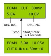
Connect the foam cutter to the DC OUT. Set up the running time, maximum current limit and the voltage. To start the foam cutter, press **START/ENTER** for more than 3 seconds. (Time is 1 to 90min, limit current is 0.05-10A, voltage is 1-25V.)
