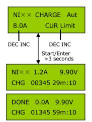
In the "Aut" mode the 680B+ charges the battery at about 1C but at no more than the maximum current you set on the second line.
