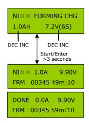
In "Forming" mode the 680B+ charges the battery at up to 1C at CC/CV mode. The function is very useful for unbalanced battery pack. Forming charge will recover battery balance status.
