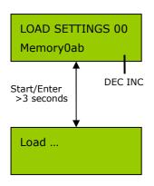
The "00" on the top line and the "memory0" on bottom line is the location you want to load dataset..
