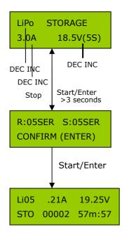
On the left side of the first line, you can set up the type of battery (LiPo, LiIo, LiFe). You can set the current and the voltage of the battery pack to be charged or discharged. The current will be used for charging or discharging the battery to reach the "storage" voltage. (Charge current: 0.05~10.0A, Voltage: 1~6 series)
