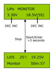
On the left side of the top line, You can set the type of battery (LiPo, LiIo, LiFe). On the second line, the cell count and the minimum cell voltage can be set. the program will monitor each cell voltage when the battery pack is discharged with external loads.
