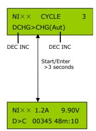
Set the charge and discharge sequence on the left and the number of cycles on the right. Set the charge current in the Charge Man or Charge Aut mode menu and the discharge current in the DISCHARGE mode menu.
