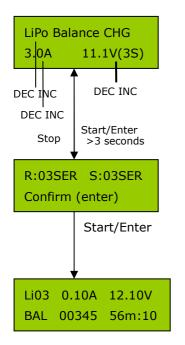
On the left side of the first line, You can set up the type of battery (LiPo, LiIo, LiFe). The values on the second line set the charge current and the voltage (cell count) of the battery pack. Press **START/ENTER** to make the value flash then press **DEC** or **INC** to adjust the value. After setting the current and voltage press **START/ENTER** again for more than 3 seconds to start the process. (Charge current: 0.05~10.0A, Voltage: 1~6 series)
