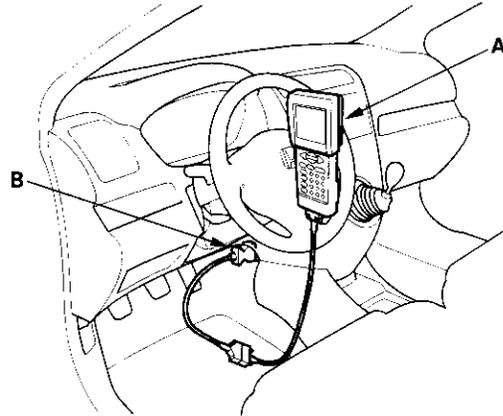
2. Turn the ignition switch ON (II), and clear the DTC(s) by following the screen prompts on the PGM Tester.
