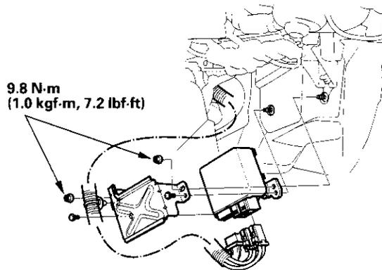
3. Disconnect the EPS control unit connectors.
