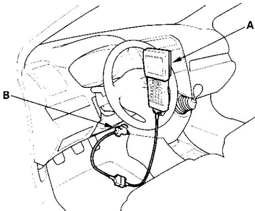
2. Turn the ignition ON (II), and follow the prompts on the PGM Tester to display the DTC(s) on the screen. After determining the DTC, refer to the DTC Troubleshooting Index.
