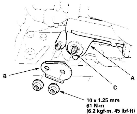
5. Install the steering stiffener B, and lightly tighten the steering gearbox mounting nuts.
