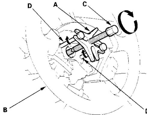
4. Remove the steering wheel puller, then remove the steering wheel nut and steering wheel from the steering column.
