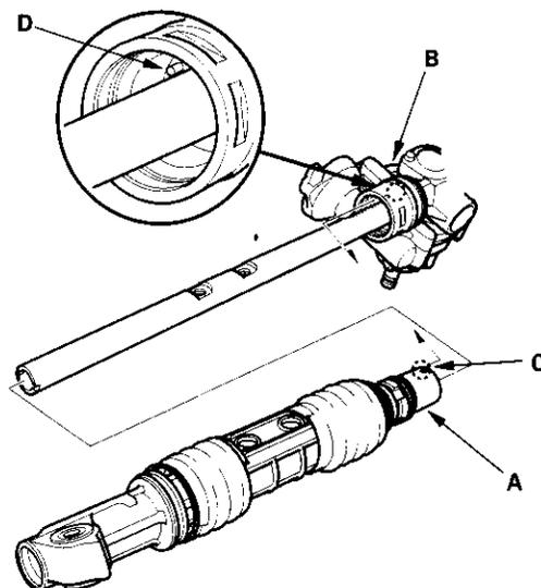
20. Tighten the lock screw (A) by hand first, then install the special tool (B) on the lock screw. Lightly tighten the lock screw. Do not tighten the lock screw to the specified torque yet.
