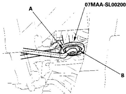
5. Remove the old sealant from rack guide screw, and apply new sealant to the middle of the threads (A). Loosely install the rack guide screw on the steering gearbox.
