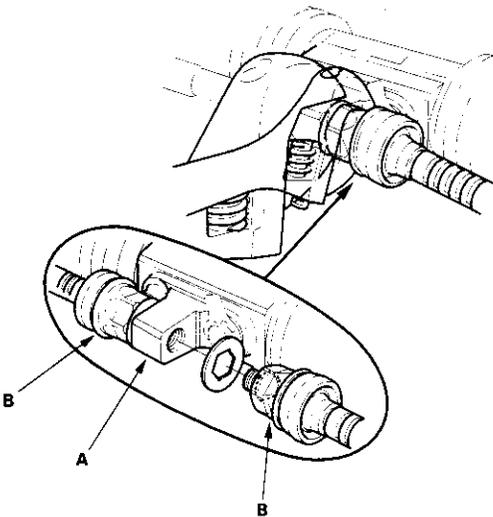
4. Remove the stop plate (A), the 12 mm flange bolts (B), the O-rings (C), and the bracket (D) from the steering gearbox.
