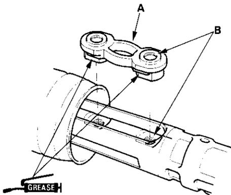
25. Center the steering rack within its stroke, and align the slider guide (A) with the holes (B) in the boot (C). Fit the slider guide to the boot by pressing around the edges of the holes securely.
