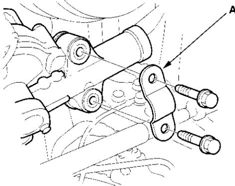
19. Remove the steering stiffener B from the right side of the steering gearbox.
