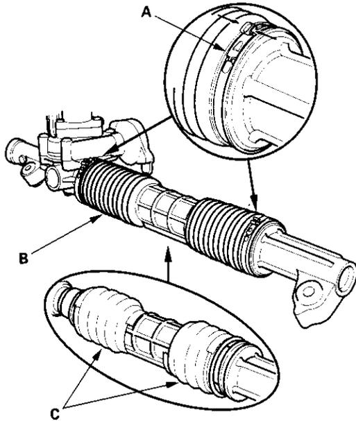
7. Attach the yoke (A) of a universal puller to the steering gearbox mounts with bolts. Securely clamp the yoke in a vise as shown. Do not clamp the steering gearbox housing in the vise.
