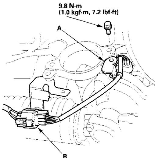
13. Install the heat shield (A).
