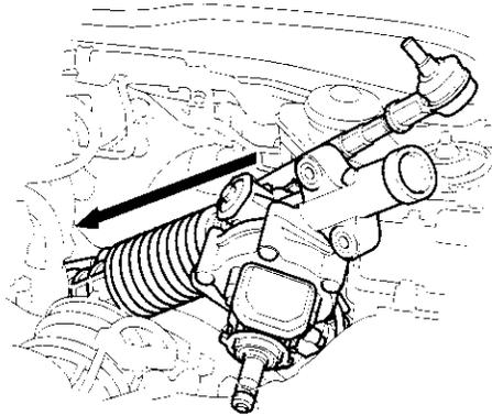
3. Install the pinion shaft grommet (A).
