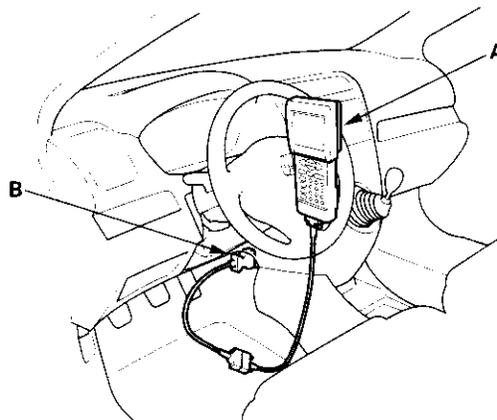
2. Short the SCS circuit to body ground using the Honda PGM Tester.
