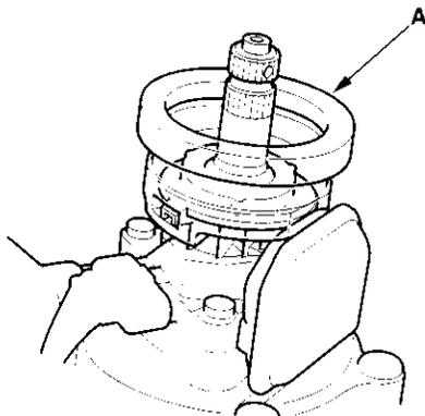
4. Insert the pinion shaft up through the bulkhead, then slip the right side of the steering gearbox housing (A) over the mounting stud (C) on the gearbox mounting bracket.
