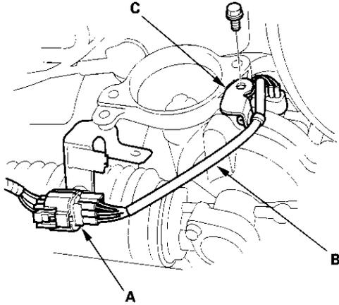
13. Remove the ground cable terminal (A) from the steering gearbox housing.
