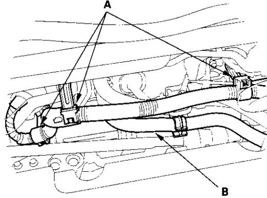
15. Remove the heater hose (B) from the bracket.
