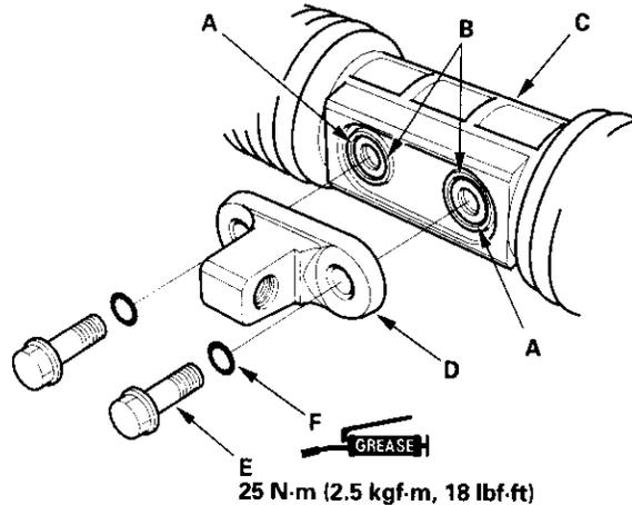
26. Before installing the bracket (D), clean the mating surface of the 12 mm flange bolts (E) and the bracket. Coat the new O-rings (F) with multipurpose grease, and install them on the 12 mm flange bolts.
