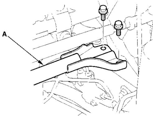
18. Remove the steering stiffener A from the left side of the steering gearbox.
