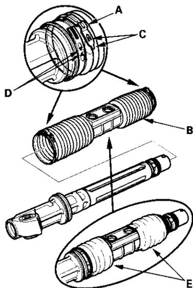
17. Compress the boot by hand, and apply vinyl tape (E) to the bellows so the boot ends stay collapsed and pulled back. Pass the boot over the rack housing so the smaller diameter end of the boot faces the steering gearbox housing.
