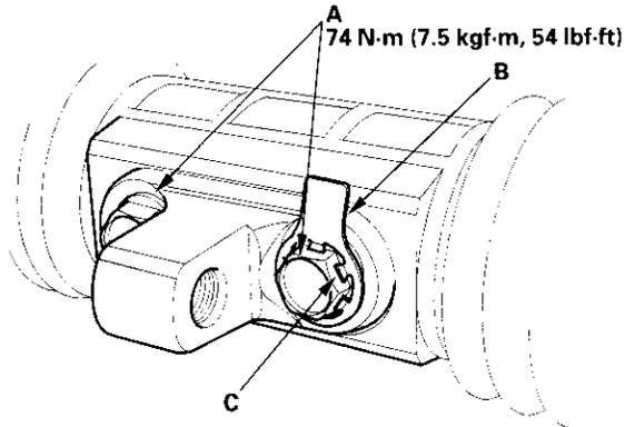
31. After tightening the 12 mm flange bolts, install a new stop plate (B) over one of the bolt heads. Be sure the tabs (C) of the stop plate are aligned with the flat surfaces of the bolt head.
