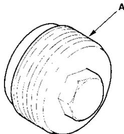
6. Tighten the rack guide screw (A) to 25 N-m (2.5 kgf-m, 18 lbf-ft), then loosen it.
