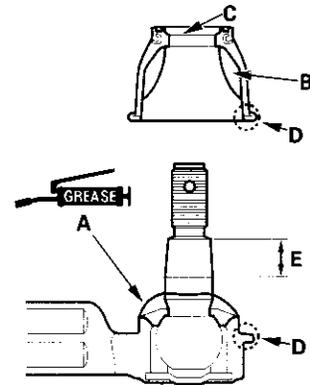
3. Pack the interior of the new boot (B) and lip (C) with fresh multipurpose grease.
