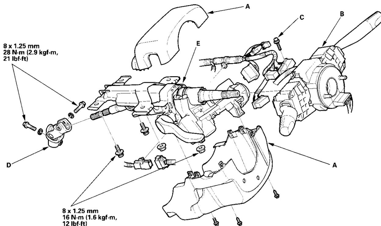
5. Disconnect the wire harness connectors from the combination switch assembly (B).
