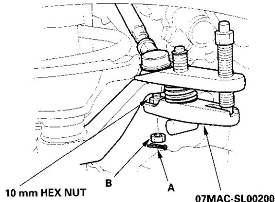
9. Separate the tie-rod ball joint and damper steering arm using the special tool (see page 18-10). Repeat on the other side of the vehicle.
