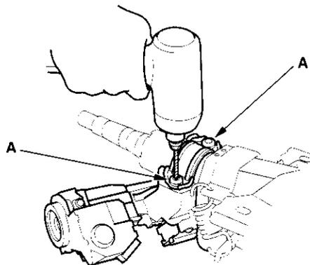
3. Remove the shear bolts from the switch body.
