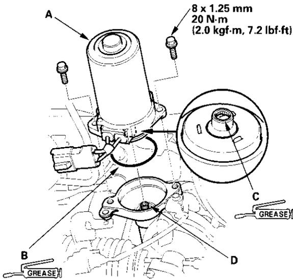
8. Apply a thin coat of silicone grease (P/N 08733-B070E) to the new O-ring (B), and carefully fit it on the motor.
