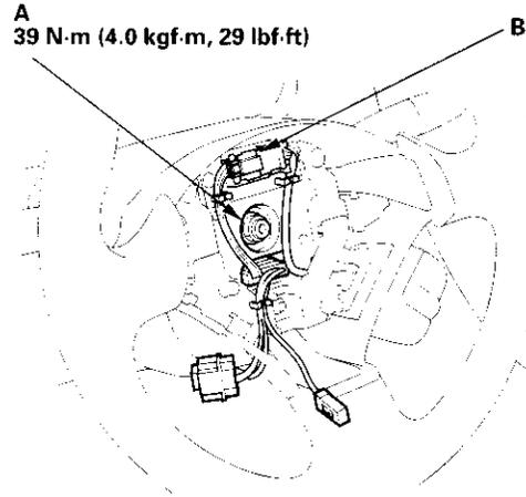
4. Connect the cruise control set/resume switch connector (B). Make sure the wire harness is routed and fastened properly.
