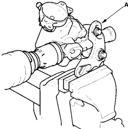
8. Install the special tool (A) on the lock screw (B) securely, then loosen and remove the lock screw from the steering gearbox housing.
