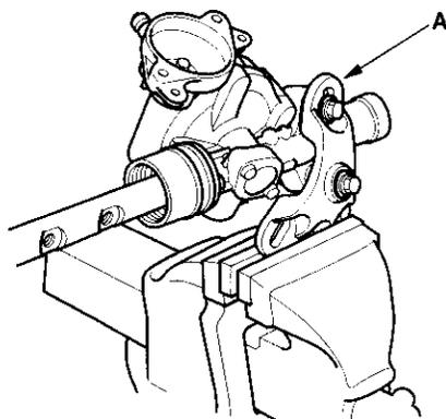
19. Push the rack housing (A) into the steering gearbox housing (B) so the notch (C) is aligned with the pin (D) on the bottom of the gearbox housing inside.
