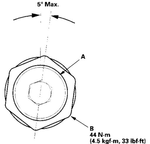
7. Retighten the rack guide screw to 6 N-m (0.6 kgf-m, 4 lbf-ft), then back it off to the specified angle.
