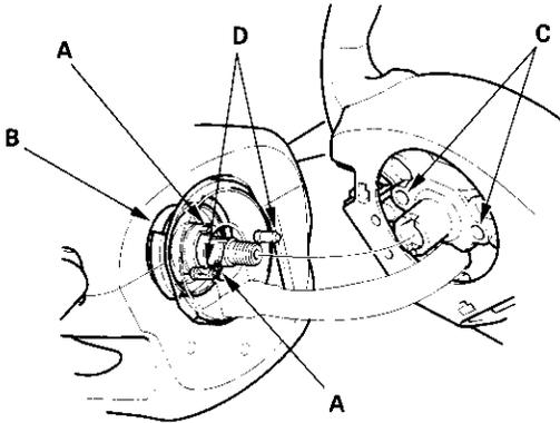
3. Install the steering wheel nut (A), and tighten it to the specified torque.
