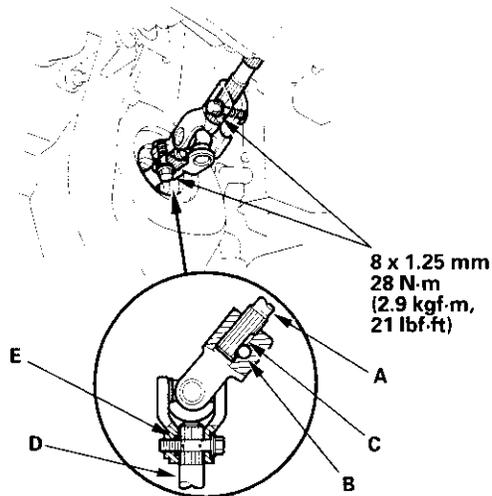
3. Slip the lower end of the steering joint onto the pinion shaft (D) (line up the bolt hole with the groove (E) around the shaft), and loosely install the lower joint bolt. Be sure that the lower joint bolt is securely in the groove in the pinion shaft.
