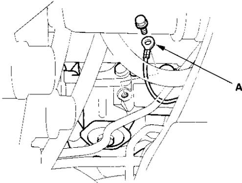
14. Remove the engine wire harness clamps (A) from the three mounting brackets.
