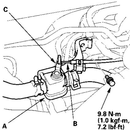
9. Reinstall the heater hose (A) on the hose bracket.
