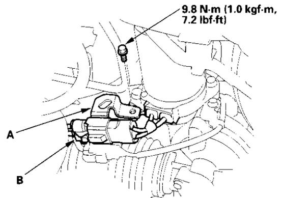
5. Remove the motor (A) from the gearbox housing.
