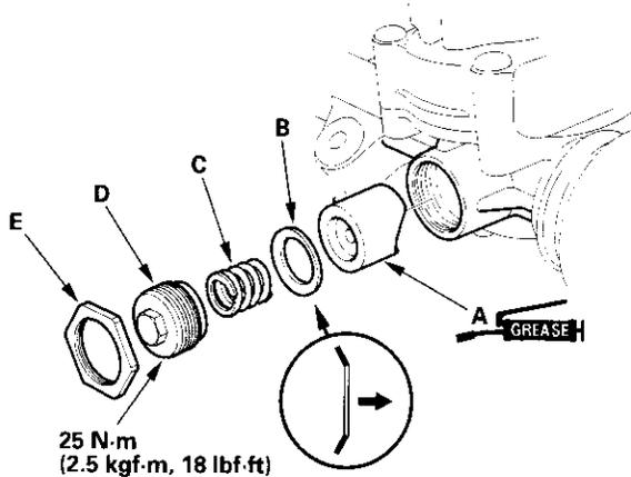
23. Install the disc washer (B) with its convex side facing the rack guide. Install the spring (C). Apply sealant to the middle of the threads on the rack guide screw (D), then install and tighten it to 25 N·m (2.5 kgf·m, 18 lbf·ft). Loosely install the locknut (E).
