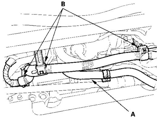
10. Install the engine wire harness clamps (B) to the three harness brackets.
