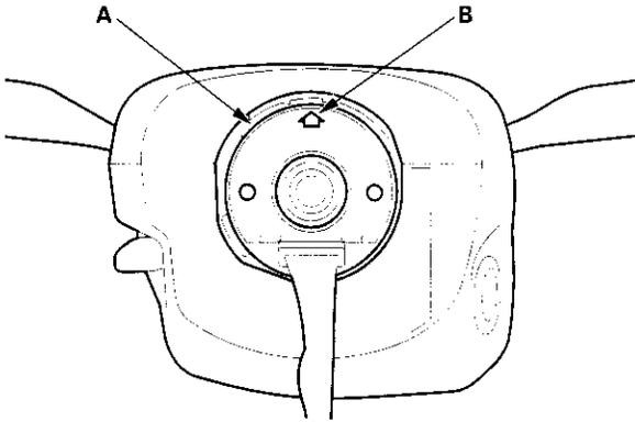
2. Position the two tabs (A) of the turn signal canceling sleeve (B) as shown. Install the steering wheel onto the steering column shaft, making sure the steering wheel hub (C) engages the pins (D) of the cable reel and tabs of the canceling sleeve. Do not tap on the steering wheel or steering column shaft when installing the steering wheel.
