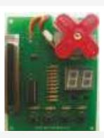
The stepper motor modules with TTL signals have been prepared for use in control experiments. The rotation of the stepper motor on the module direction, change of speed, different designs, such as displaying the number of steps in the 2x7 segment display can be improved according to the changing speed.
