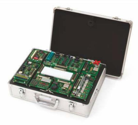
ES130 Trainer kit with PIC 8, 14, 18, 28 and 40-pin PDIP package with the type of PIC or choose from depending on your PC's USB port and to send electrical signals from the RS232 COM port programs will be able to.
