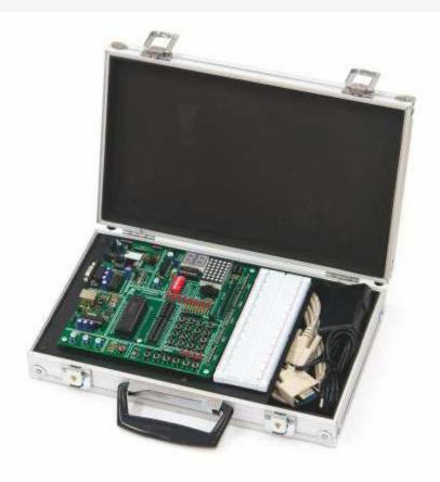
PIC PROG DEKA V5 sets of experiments with 18, 28 and 40-pin PDIP package type with your PC's USB PIC with electrical signals to send to the port programs will be able to. Your program is finished bits PIC programs that automatically run will begin.
