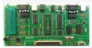
On the programmer circuit is different pin number where the module connector and socket that can be connected with other modules can be placed in PICs. As a user level, from beginners to professional design that is suitable for microcontroller programming and training at all levels. Microcontrollers on the main programming module as optional USB or serial port (RS232) is programmed by means of.
