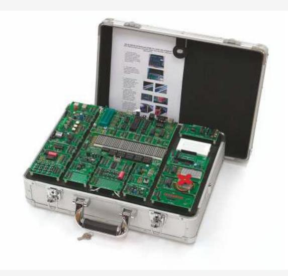
Atmel AVR microcontroller training Kit (ES120.01) Advantages: at all levels in the preparation of this set of experiments aimed to benefit the user. As well as perform simple operations such as quenching of a button will be lit with LED AVR programming beginner's first try, try more complex operations, such as a user's advanced RF communications possible. Also Atmel AVR (ATtiny2313) of samples can be tested on this set of programs in programming books.
