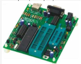
ATMEL 8051 V1 are given, together with the programming card: PROG 8051 V1
