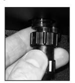
**8** Attach the two (2) Epi White Light Cable Connectors (smaller connector) into the keyed connections on both sides of the ceiling in the cabinet.
