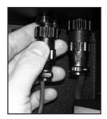
**9** Connect the Camera/Computer FireWire Interface Cable to the back of your GL212 PRO Imaging Cabinet.
