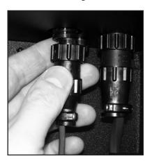
**5** Use the retaining clips on the right side of the cabinet to retain the White Light Transilluminator Connector Cord.
