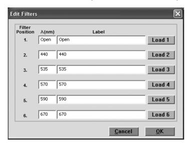
**4** Click the Load button of the filter position you want to install. The Emission Filter Wheel moves to the correct loading position.
