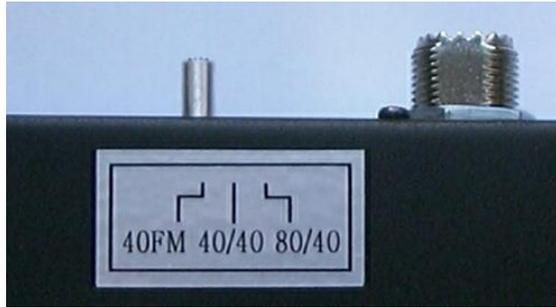
Before You install Your new CB radio, You should preset the country switch on the rear side of the radio according to the local authority requirements. Because this radio is used in most cases by truck drivers in central and western Europe, it comes programmed with the center switch position 40/40 channels. If You are in a country where this setting should not be allowed,
