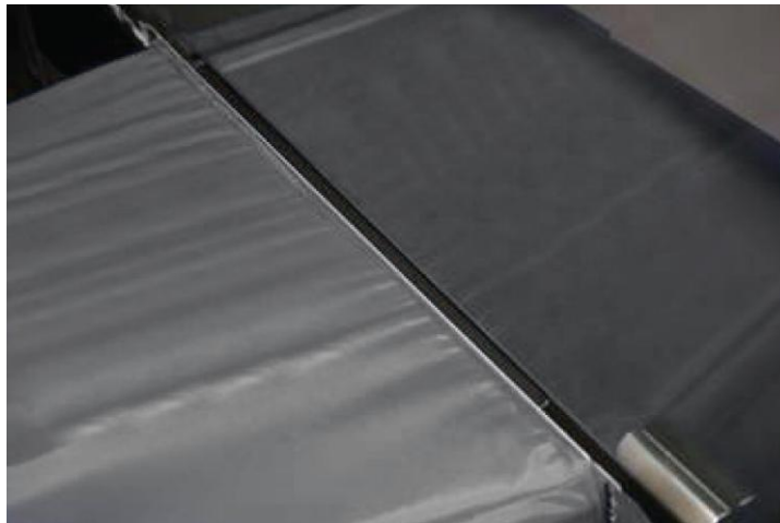
Figure 29: Lower Sash of Cabinet Until it Rests on Foam Lip of Hood Frame
