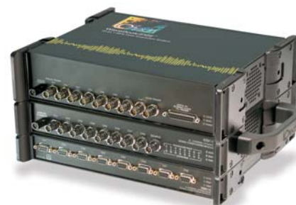
WaveBook system with 8 strain inputs and 8 accelerometer inputs
