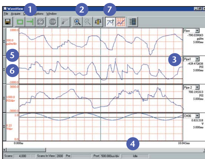
Scope Mode allows you to display any eight of the WaveBooks' channels
