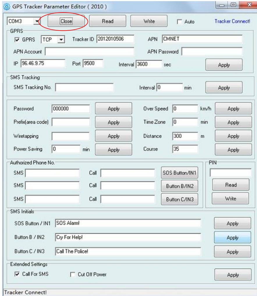
5) Switch on MT210, wait until the two LED indicators stop flashing and keep ON status. As soon as they connect successful, all the buttons are visible and the status bar will show 'Tracker Connect!'. First click "Read" to read setting from device, when all the parameter read out, you can put in the parameters you need.
