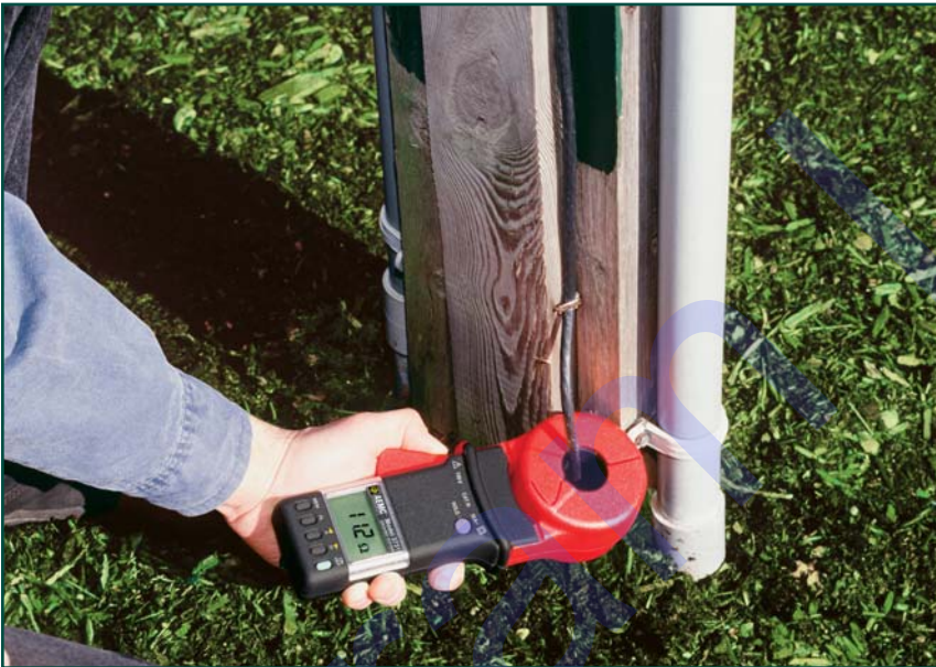
Model 3731 performing a ground rod resistance check.
