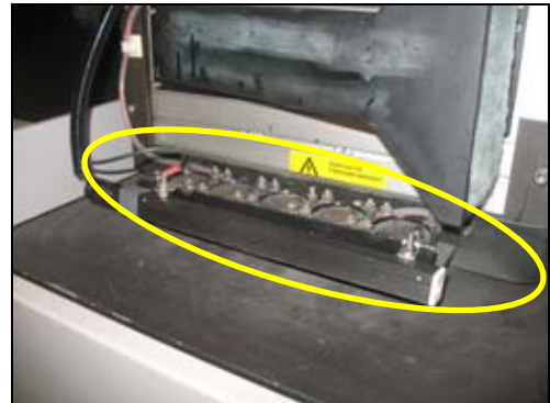
Figure 2: Left Ionizer Unit
