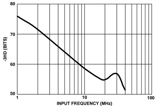
FIGURE 10. THIRD HARMONIC DISTORTION (3HD) vs INPUT FREQUENCY
