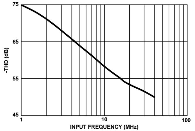
FIGURE 6. TOTAL HARMONIC DISTORTION (THD) vs INPUT FREQUENCY
