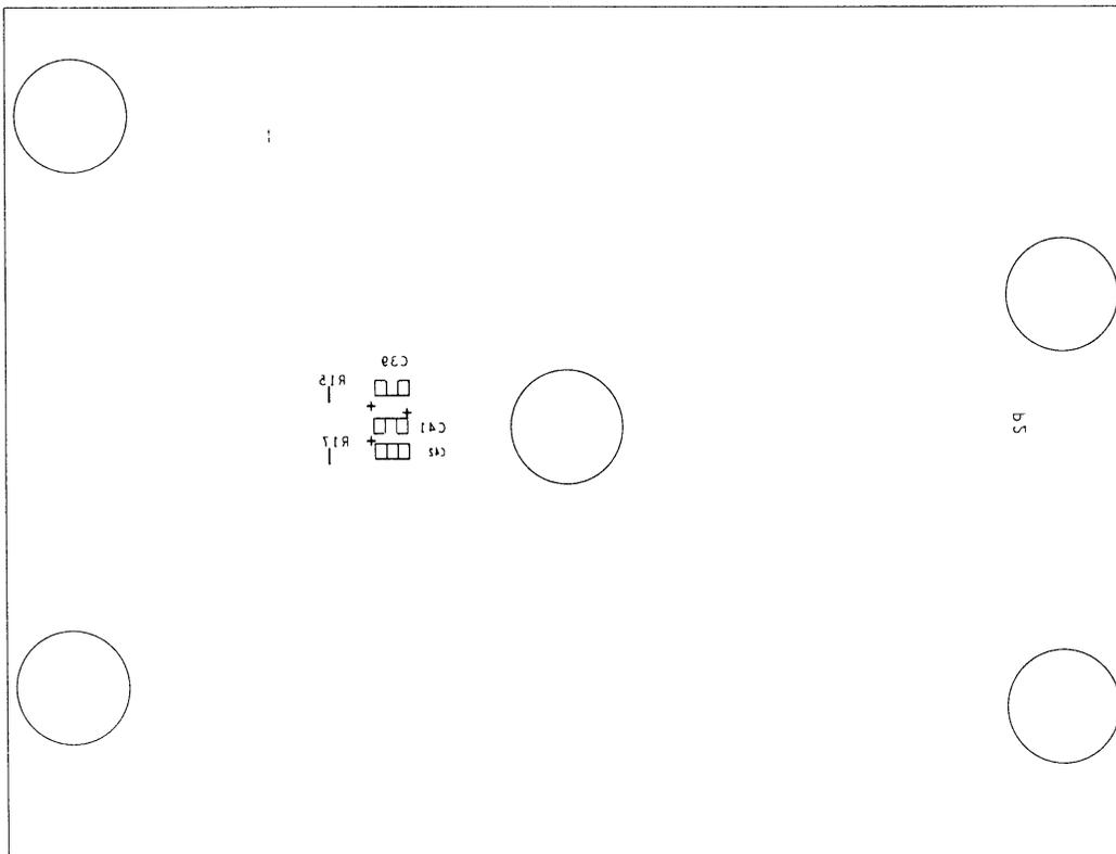
FIGURE 16. HI5905EVAL2 EVALUATION BOARD PARTS LAYOUT (FAR SIDE)
