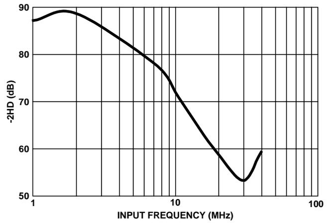
FIGURE 8. SECOND HARMONIC DISTORTION (2HD) vs INPUT FREQUENCY
