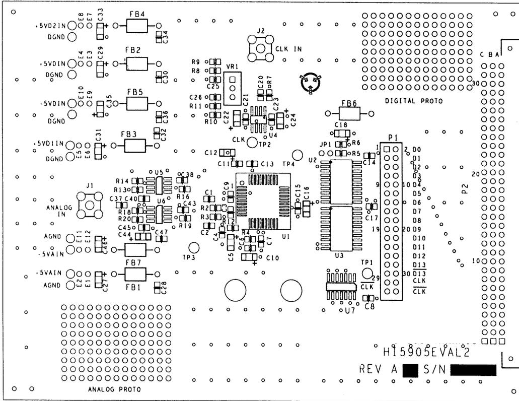
FIGURE 11. HI5905EVAL2 EVALUATION BOARD PARTS LAYOUT (NEAR SIDE)
