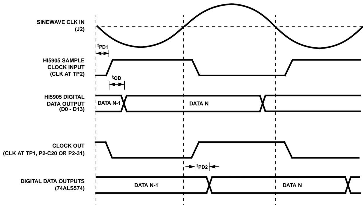
**FIGURE 3. EVALUATION BOARD CLOCK AND DATA TIMING RELATIONSHIPS**
