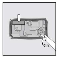
[2] Install a battery and turn the letter selector to the desired letter (="house code").
