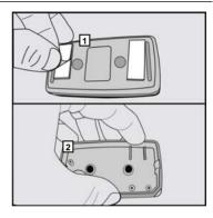
[3b] (1) Place the double-sided tape vertically at both ends of the back.
