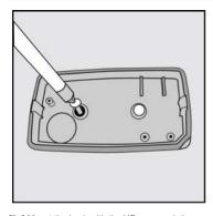
[3a] Mount the back with the UP-arrow pointing upward. Install the screws through the two mounting points.
