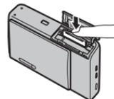
Push the **xD-Picture Card** into the slot and then slowly remove your finger. The lock is released and the **xD-Picture Card** is pushed out.
