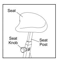
turns to loosen it. Next, pull the seat knob, raise or lower the seat post, and then release the seat knob. Move the seat post up and down slightly until it locks into position. Then, tighten the seat knob. CAUTION: Make sure that the pin on the seat knob is inserted into one of the adjustment holes in the seat post. Do not rest the seat post on top of the pin on the seat knob.
