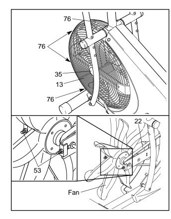
If the Belt (22) needs to be adjusted, loosen the right Guard Fastener (not shown). To tighten the Belt, turn the M6 Nuts (53) clockwise; to loosen the Belt, turn
