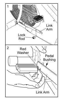
gers as shown. Be careful not to pinch your fingers. Next, slide the link arms onto the pedal bushings. Move the link arms up and down slightly to make sure that they are fully seated on the pedal bushings. CAUTION: Make sure that the link arms are fully seated on the pedal bushings. If the link arms are not on the pedal bushings, they may slip off during use, resulting in injury to the user.
