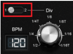
Figure 3: the switch in the red box appears when the Mode is set to PAR . From there, you can select a different Division factor for the rows 1 and 2
