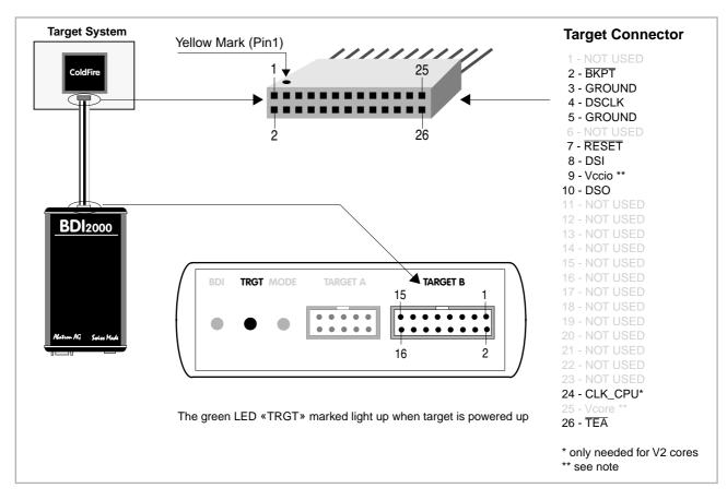
The target CPU clock is only needed for older V2 cores (MCF5204, MCF5206(e) and MCF5272) because DSCLK and DSI have to change synchronous with the CPU clock. For all other cores, BDM communication can be asynchronous to the CPU clock and therefore this signal is not needed.
