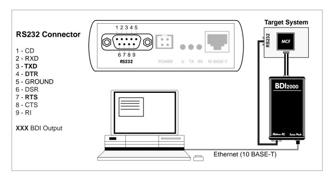
The configuration parameter "SIO" is used to enable this serial I/O routing. The BDI asserts RTS and DTR when a TCP connection is established.
