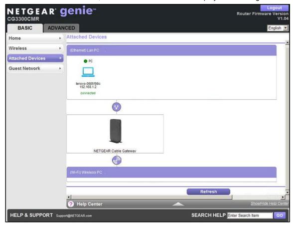
Wired devices are connected to the gateway with Ethernet cables. Wireless devices have joined the wireless network.
