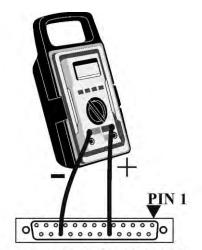
REAR OF CONNECTOR, CONNECT PINS 18 AND 23 FOR 0-2 VOLT OUTPUT. JUMPER ON BOARD IS AT "V" Figure 1
